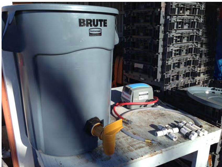
Brewer consists of 1) 45 gallon garbage can with spigot, 2) quick release air line, 3) pvc diffuser, 4) heavy duty air pump.
