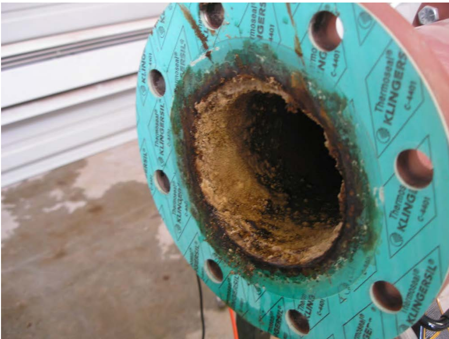
Note buildup of scale at pipe as water enters the Zetacore unit (untreated water)
