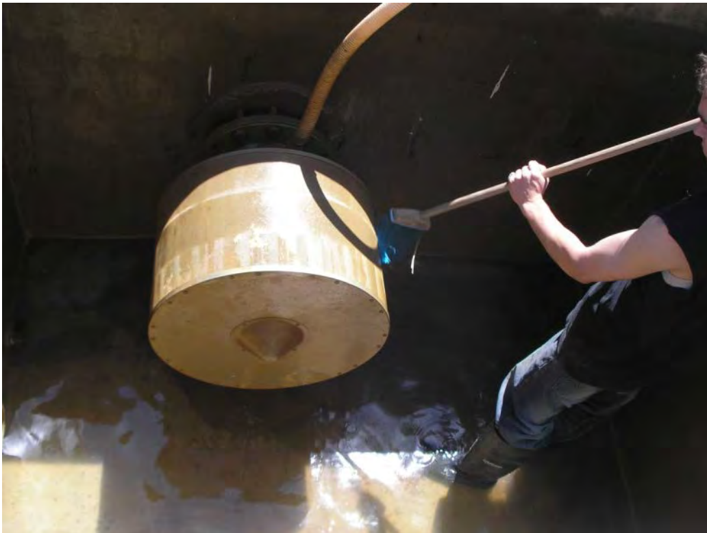
Cleaning the spinner is critical
