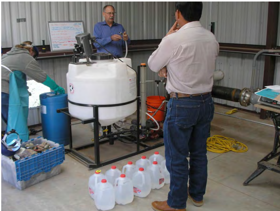
Injector pump with tank- note blue drum of hydrogen peroxide
