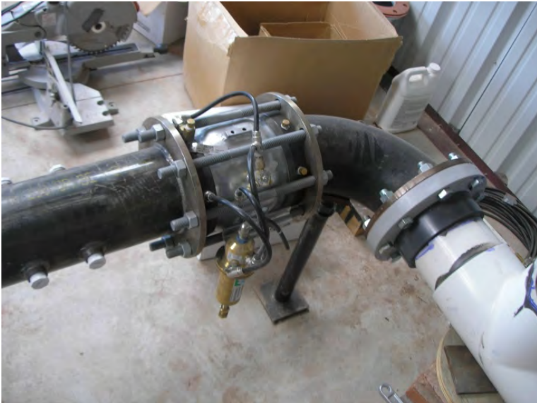
pressure reducing valve- reduces pressure from 40 psi to 20 psi
