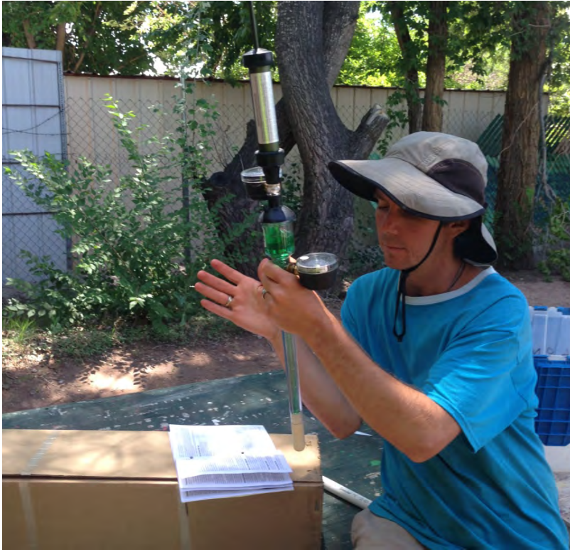
Prepping tensiometers for placement in field
